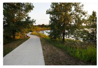
for the required width. AASHTO guidelines recommend a minimum width of 10 feet, and they can have various surface types such as concrete, asphalt or crushed limestone.
